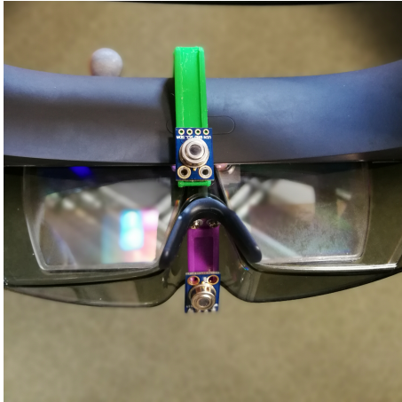
Figure 6: Thermal sensors embedded on HoloLens with 3d-printed adjustable components for task assistance.
