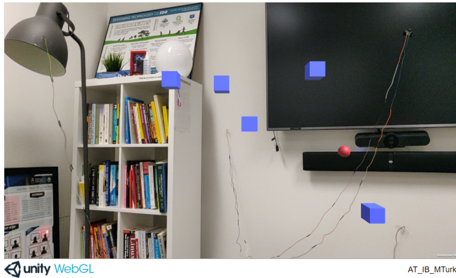
Figure 5: Image of the WebGL application running on a web browser window used in study 2. The application is presenting a background image with physical LEDs and is overlaid with virtual blocks.
